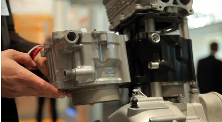
*The aluminium cylinder casing (left) next to its composite replacement mounted in the engine (right).*
